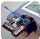
Liquids containment well prevents chemicals from spilling.
