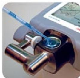
Liquids containment well prevents chemicals from spilling.
